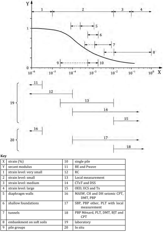
Figure F.1 — Typical strain ranges for common geotechnical constructions and tests (see Atkinson and Sällfors, 1991)
